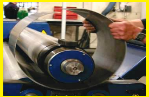
ROLLING AND BENDING (EVEN 500 BHN PLATES.)
